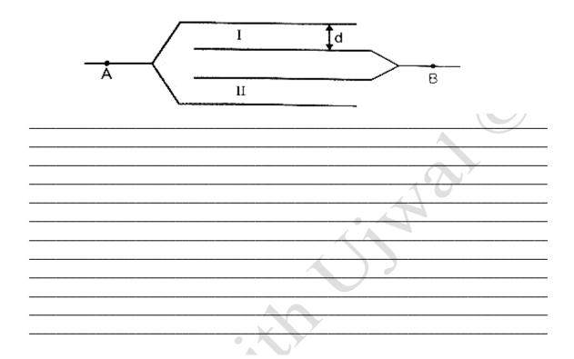
What is the capacitance of arrangement of a 4 plates of area A at distance d in air in 10. figure? [Ans.  $3\varepsilon_0 A/d$ ]
