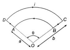
A circular segment of radius 10cm subtends an angle of 60° at its centre. A current of 9A 16. is flowing through it. Find the magnitude and direction of the magnetic field produced at [Ans.  $9.42 \times 10^{-6}$  T] the centre.
