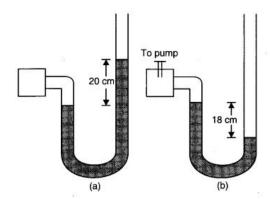
The liquid used in the manometers is mercury and the atmospheric pressure is 76 cm of mercury.
