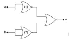
Analyse the action of the gates (1) and (2) and identify the logic gate of the complete circuit so obtained. Give its symbol and the truth table.
