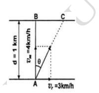
In the figure,  $\vec{v}_m$  and  $\vec{v}_R$  are the velocities of man and river. Clearly  $\vec{v}$  is the resultant of these velocities. If the man begins to swim along AB, he will be deflected to the path AC by flowing river.
