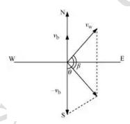
When the boat is stationary, the flag flutters along NE direction. This shows that velocity of the wind is along NE direction. When the boat moves the flag flutters along the direction of relative velocity of wind w.r.t. boat. Thus  $\mathbf{v}_{\mathbf{w}} = \mathbf{O}\mathbf{A} = \text{wind velocity} = 72\text{km/h}$  due NE direction.
