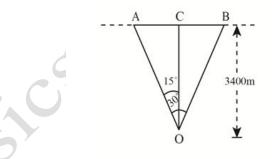
Then  $\tan 15^\circ = x/3400$ Or  $x = 3400 \tan 15^\circ = 3400 \times 0.2679 = 910.86m$ Speed of aircraft = 910.86m/5s = 182.2 ms<sup>-1</sup>.
