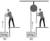
Sol. In mode (a) the man applies force equal to 25kg wt in the upward direction. According to Newton's third law of motion, there will be downward force of reaction on the floor. Therefore, total action on the floor buy the man = 50kg wt 25 kg wt = 75 kg wt =  $75 \times 9.8N = 735N$ In mode (b) the man applies a downward force equal to 25 kg wt According to
