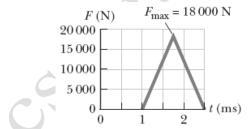
From this curve, determine (i) impulse delivered to the ball (ii) force exerted on the ball (iii) the maximum force on the ball.
