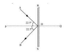
The horizontal components of velocity are to be considered for imparting impulse as vertical components are in the same direction thus impulse in the vertical direction is zero.
