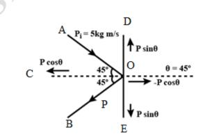
Initial momentum is along AO. It has two rectangular components: p cos 45° along CO and p sin 45° along DO. Final momentum p is along OB. It has two rectangular components: p cos 45° along OC and p sin 45° along OE Change in momentum along vertical direction = final momentum – initial momentum  $= p \sin 45^{\circ} - p \sin 45^{\circ} = 0$
