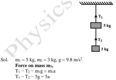
Force on mass m<sub>1</sub>,  $T_1 - T_2 - m_1g = m_1a$   $T_1 - T_2 - 5g = 5a$   $T_1 - T_2 = 59.0 \text{ N}$ Force on mass m<sub>2</sub>  $T_2 - m_2g = m_2a$  $T_2 = m_2 (g + a) = 3(9.8+2)$   $\begin{array}{l} T_2 = 35.4 \\ T_1 = T_2 + 59.0 \\ \text{or} \ T_1 = 35.4 + 59.0 = 94.4 \ \text{N} \end{array}$
