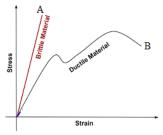
Stress strain curve of brittle and ductile materials can be shown in the given figure. In the figure curve A represents the brittle material and B represents ductile material.
