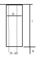
Suppose the length of the loaded wire increases from l to  $l + \Delta l$  and its diameter decreases from D to  $D - \Delta D$ .
