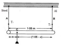
Suppose the mass m is suspended at distance x from wire A. let  $T_1$  and  $T_2$  be the tensions in the steel and aluminium wires respectively
