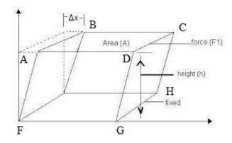
Consider a rectangular block whose lower face EFGH is fixed. Let a rectangular force F be applied on the upper face ANCD of the block in direction shown. The force provides a shear stress which displaces the upper face through a small distance  $AA' = \Delta L$ .
