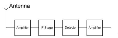
The basic description of all the parts of the AM receiver is as follows Receiving antenna – A receiving antenna functions opposite to a transmission antenna and receives the amplitude-modulated wave and converts it into electric current and feeds it to the amplifier.
