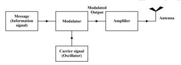
The block diagram shows the process of modulation. The low frequency message modulating signal and high frequency carrier wave obtained from an oscillator are given as inputs to the modulator. The modulator now produces the modulated output. This modulated output is amplified by an amplifier and then transmitted through the antenna.
